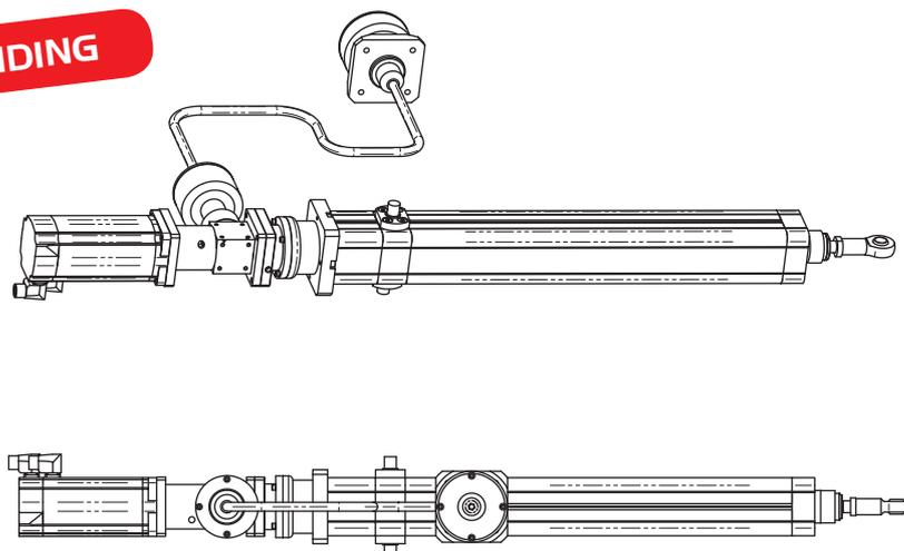
AZIONAMENTO REMOTATO CON MOTORE AUSILIARIO / REMOTE AUXILIARY MOTOR DRIVE
