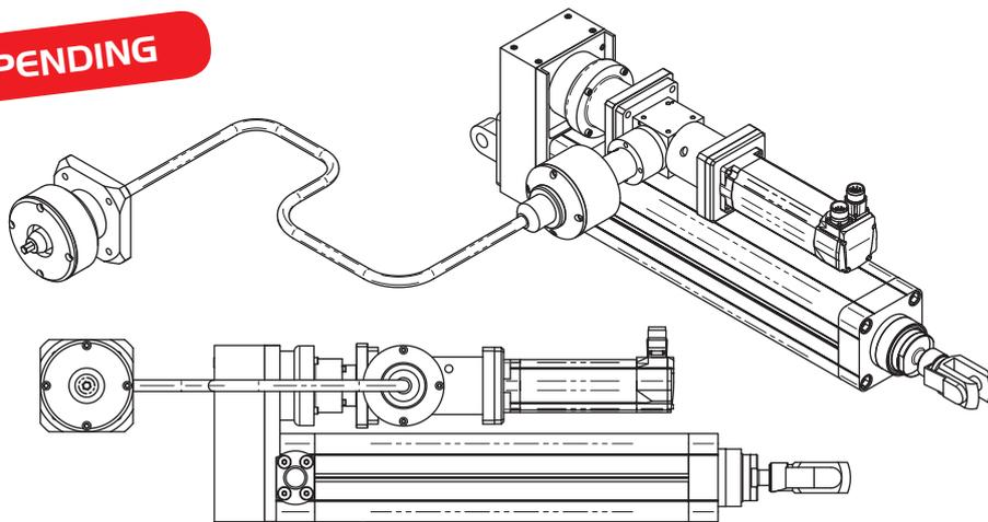
AZIONAMENTO REMOTATO CON MOTORE AUSILIARIO / REMOTE AUXILIARY MOTOR DRIVE
