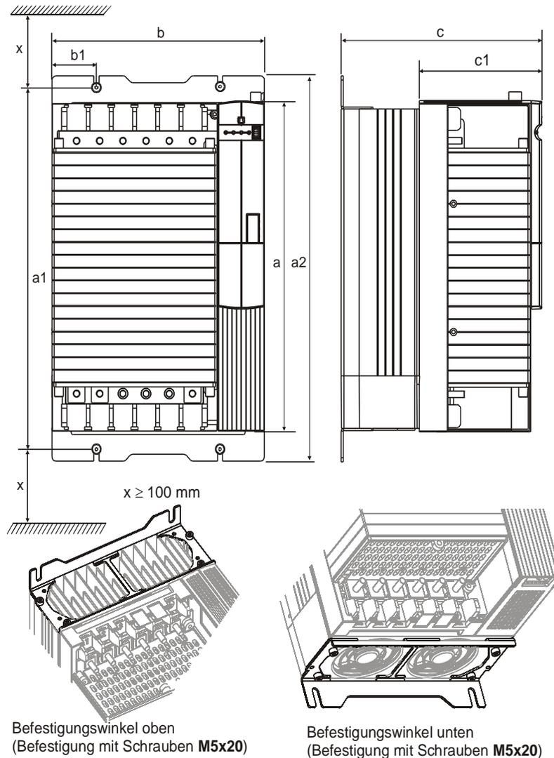
Assembly is done by screwing the two fixing brackets to the heat sink of the device and the assembly panel. The devices are provided with fixing brackets, which are fitted using four thread-cutting screws. The dimensions of the device and the installation dimensions are those of the standard device without optional components and are given in millimeters.
