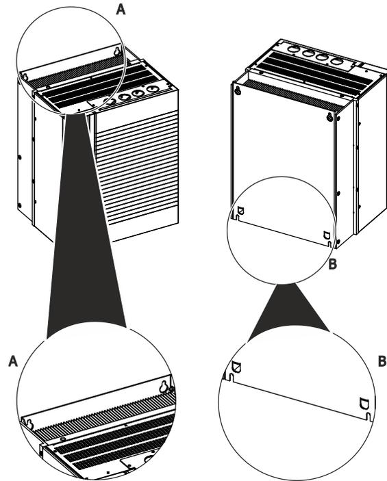
Assembly is done by screwing the back wall of the device to the assembly panel. The dimensions of the device and the installation dimensions are those of the standard device without optional components and are given in millimeters.
