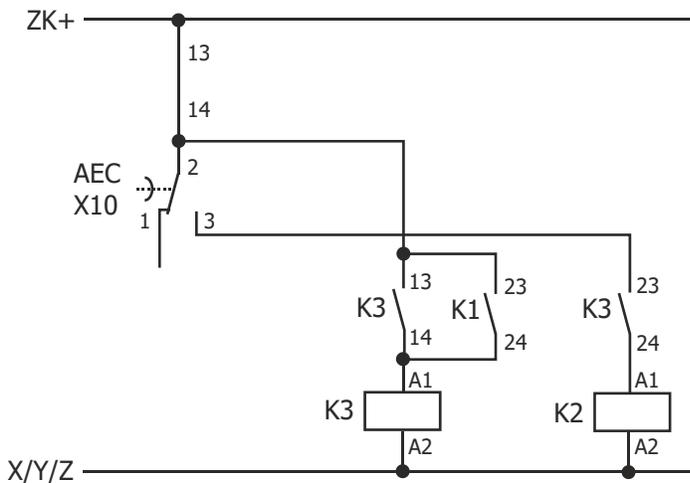
Mains contactor K2 must be designed for the maximum expected braking power of the drive.
