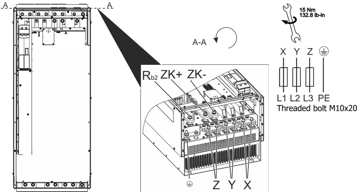
**Figure 8-4: Connection of mains unit precharger , size 8**
