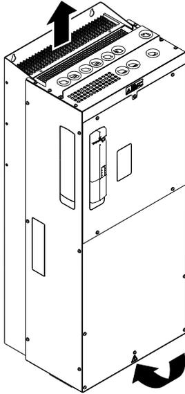
For cooling air-cooled mains units, air is taken in through openings in the bottom plate. The air coming from below heats up and escapes through openings in the top of the case. The illustration shows the air flow from below in the case of a device of size 8.
