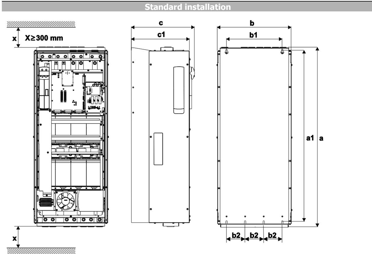
The diameter of the fixing holes is 9 mm.
