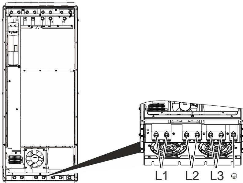
**Figure 8-5: Connection of mains unit sine unit, size 8**
