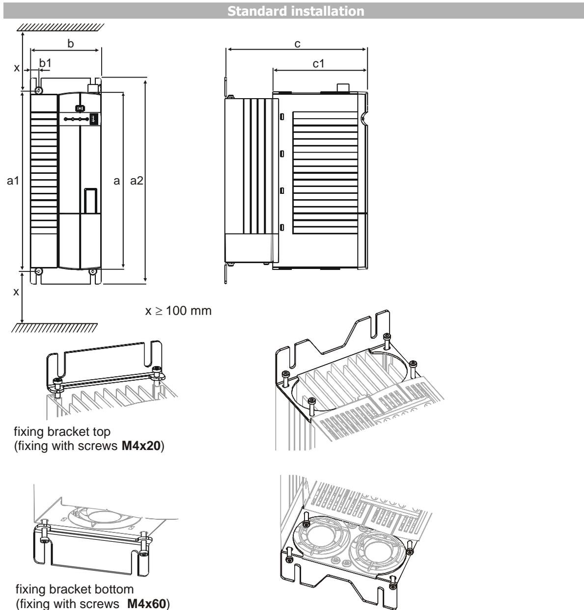
Assembly is done by screwing the two fixing brackets to the heat sink of the device and the assembly panel. The devices are provided with fixing brackets, which are fitted using four thread-cutting screws. The dimensions of the device and the installation dimensions are those of the standard device without optional components and are given in millimeters.
