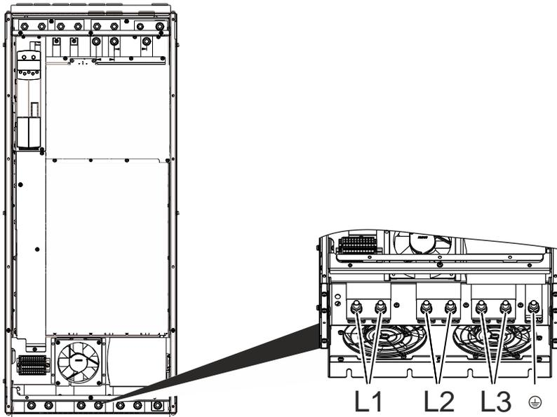
**Figure 8-9: Connection of feed-back unit line choke, size 8**
