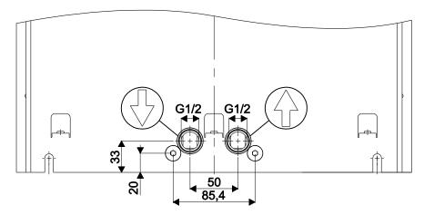
Bottom coolant connection ports:
