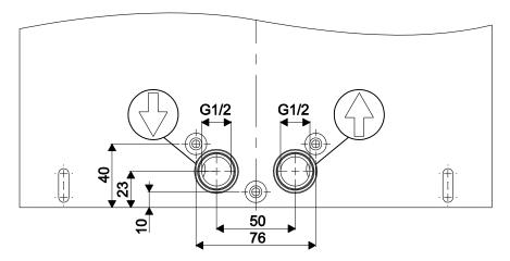
Bottom coolant connection ports:
