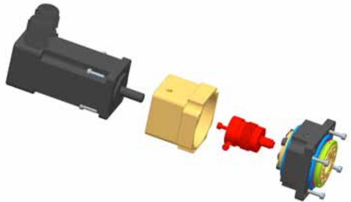
Fig.5.4.1b: Shaft connection by using flexible coupling / Spojenie hriadel'ov pomocou pružnej spojky
