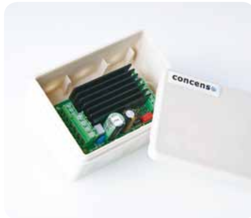
C2-20-BOX-000-000000 (box version) 102 x 73 x 47 mm (L x W x H)
