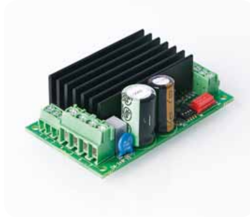
C2-20-PCB-000-000000 (board alone) 73 x 43 x 25 mm (L x W x H)
