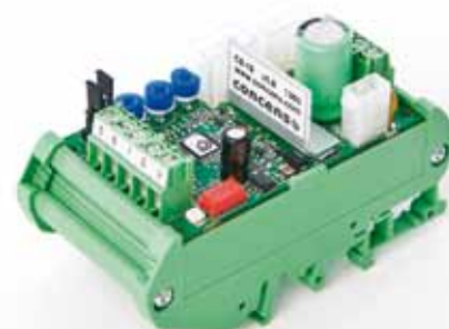
C2-10-DIN (DIN rail version) 90 x 46 x 56 mm (L x W x H)
