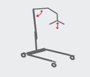
Personal lifts are used as auxiliary equipment to lift people in and out of beds, wheelchairs and toilet/shower chairs. Before the lift, the person is arranged in a sling supplied with girths and belts attached to the cradle of the personal hoist. The distance between the legs can be extended to increase stability.
