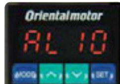
Alarm Code 10 Indication
