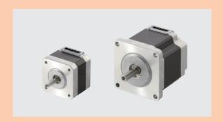
This is a high torque and low vibration stepper motor with a basic step angle of 0.72° (resolution of 500 steps per revolution).
