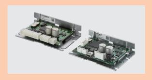
These are DC power supply input drivers for stepper motors. 2-phase stepper motors (bipolar drive) and 5-phase stepper motors are available. Using the microstep drive function for a low-vibration driver reduces vibration and noise.
