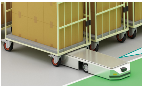
Transportation robots for flat, transportable masses can be designed
