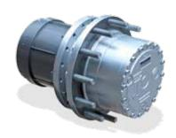
This complete mechatronic solution from Bonfiglioli was originally conceived for use on self-propelled crop sprayers. It can, however, also be applied to other types of new-generation hybrid agricultural vehicle capable of integrating electrical power with a mechanical transmission and weighing between 7 and 20 tons. It incorporates a high-power electric motor, instead of the conventional hydraulic motor, and a braking system.
