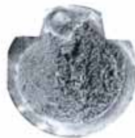
Fig.2: fatigue problem caused by torsion
