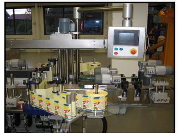
All the same performances obtainable from the single head labelling can be transferred to the multi-axis labelling, the solution consists of a SW1 for each labelling head (max 8) connected through RS485 interface to a VT series HMI.
