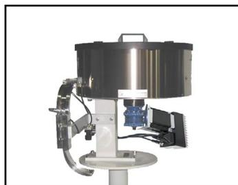
Complete solution, stand alone (with HMI), can be interfaced to PLC through fieldbus for the management of caps orientation process:
