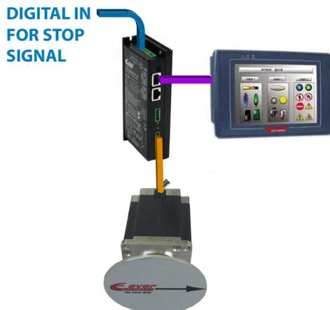
The drive commands the motor according to the programmed cycle motion and it performs a precision stop each time the digital stop signal is activated (for example, mick finder or label presence digital sensor closure). After stop signal activation, a number of steps can be configured within the drive and can be managed by HMI or PLC like all other motion parameters.
