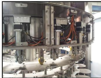
Full digital "Plug & Play" solution for linear and rotative filling machines control.
