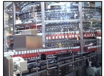
The solutions for rotary labelling machines control allow high speed and high precision labelling of bottles and containers having different shapes and size. In addition to the management of more synchronous applicators (from one to four heads per machine), solutions are available for electronic cam management of the carousel which transport and direct the products, consisting of a maximum 32 plates.
