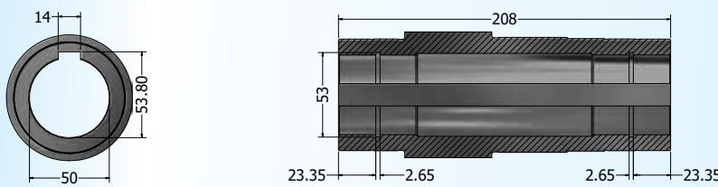
The standard hollow shaft diameter for a FFA78 is 50mm
