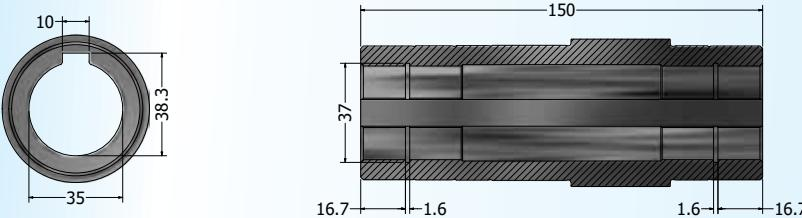
The standard hollow shaft diameter for a FFA48 is 35mm
