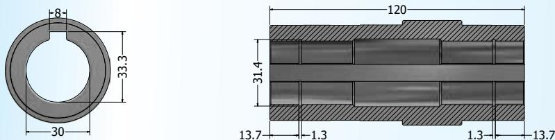
The standard hollow shaft diameter for a FFA38 is 30mm
