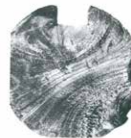
Fig.3: typical fatigue fracture
