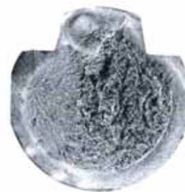
Fig.2: fatigue problem caused by torsion
