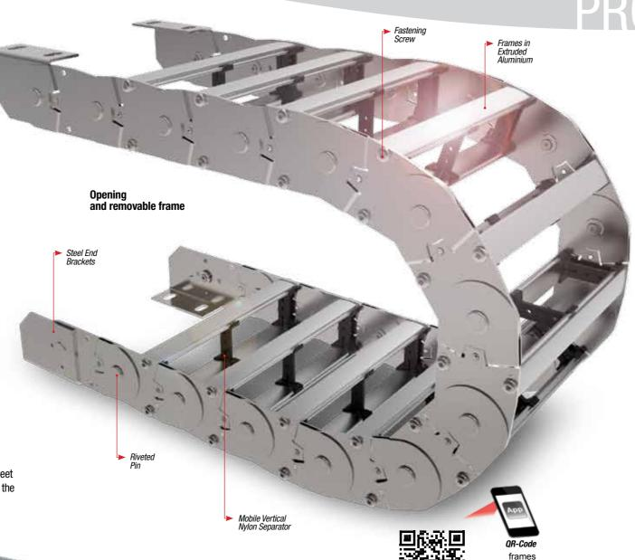
The "L" series is available in four versions and offering several configurations: open with steel rods, fully enclosed with aluminium covers, aluminium drawplates and customised crosspieces. Thanks to many types of spacers and separators, Brevetti Stendalto offers endless possibilities to customise the interior layout.
