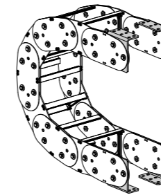
Fig. A Chain fixed outside the radius. (Fig A) See end brackets mounting variations page 31.
